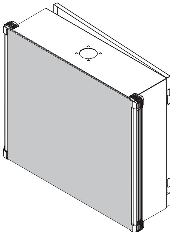
The front plate cutout for the OI device must be made by the customer. Follow the OI device mounting instructions.
