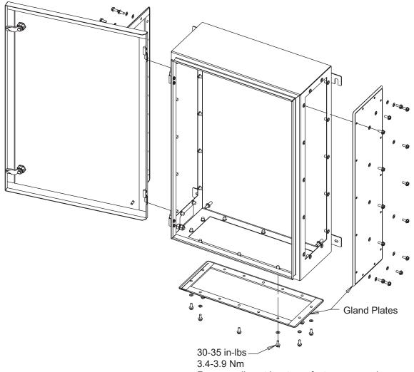
For grounding at least one fastener on each gland plate must not have a nylon washer under the head.
