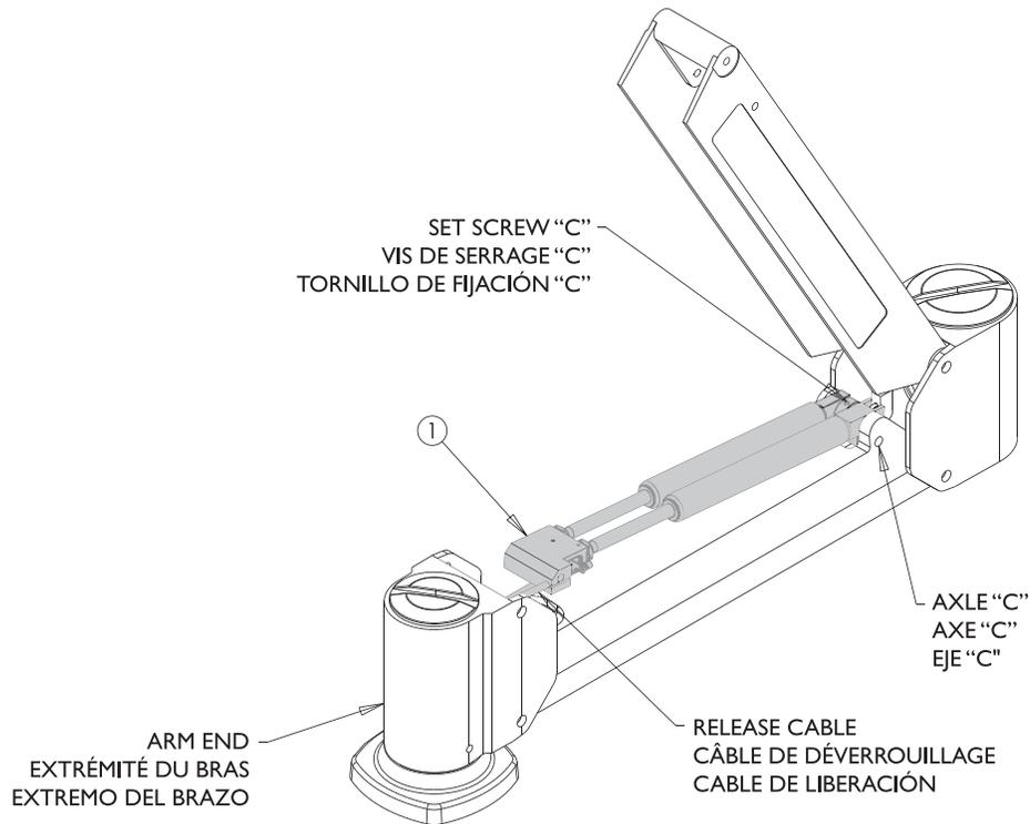
3. Remove axle "B". A light tap with a drift should be sufficient. Raise the arm top half (cover) to about 45°, and tie it off in that position so that it will be out of the way for servicing.
