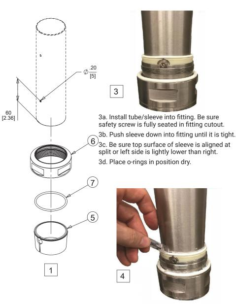
4a. Lube top surface of both o-rings (the surface the nut will contact).
