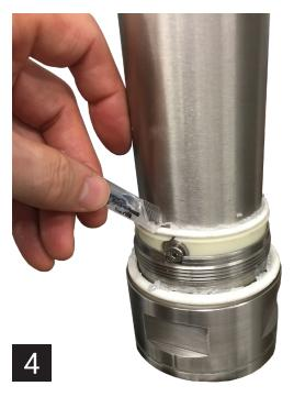
Lube top surface only of both o-rings (the surface the nut will contact)
