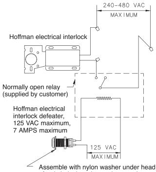
of switch; lockwasher and nut on the inside of the door. (see defeater mounting hole detail)
