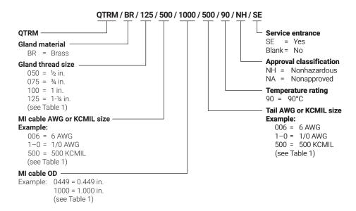
Example: Sized-up QuickTerm kit required for 1/3/0-621, single conductor # 3/0 AWG cable to use a 350 kcmil tail is:
