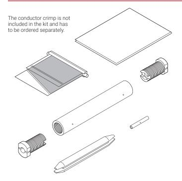
The kits nVent RAYCHEM CS-150-xx-PI are designed to connect a PI cold lead cable to a polymer insulated (PI) series heating cable as well as to splice two PI heating cables. The kit employs a two component silicone compound to provide durable and flexible moisture proof encapsulation.
