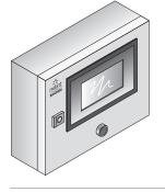
The Remote User Interface Terminal (NGC-UIT3-ORD-R) is a stand-alone display for use with the nVent RAYCHEM NGC-30 panel. The NGC-UIT3-ORD-R is mounted remotely (in a nonhazardous location). Like the NGC-UIT3-EX, it has a 7 inch x 5¼ inch (17.5 cm x 13.3 cm) LCD color display with touch-screen technology, and provides an easy user interface for programming without using keyboards. It is rated NEMA 4 (IP 65), and must be mounted in a nonhazardous indoor or outdoor location.
