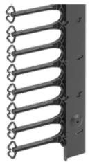
Fingers separate, support and manage cable. Bracket mounts on either left or right side of 700- and 800-mm cabinets between the frame and the rack angle to create vertical wiring space. Bracket has RAL 9005 black polyester powder paint finish. Fingers are molded black plastic. Mounting hardware included. NOTE: Refer to the table to calculate the number of reducing brackets required.
