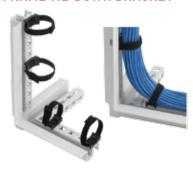
The PROLINE Frame VELCRO® Tie-Down Bracket provides an easy means to secure and bundle cables using any of the frame's rectangular holes. The bracket can be positioned parallel or perpendicular to the frame and needs no tools to install—just push into any hole and twist to fasten. Proper bend radius is easily maintained with the flexible Velcro tie-down, plus it provides easy initial and future cable installations. Bracket is made of a durable plastic. Both tie-down and bracket are black.
