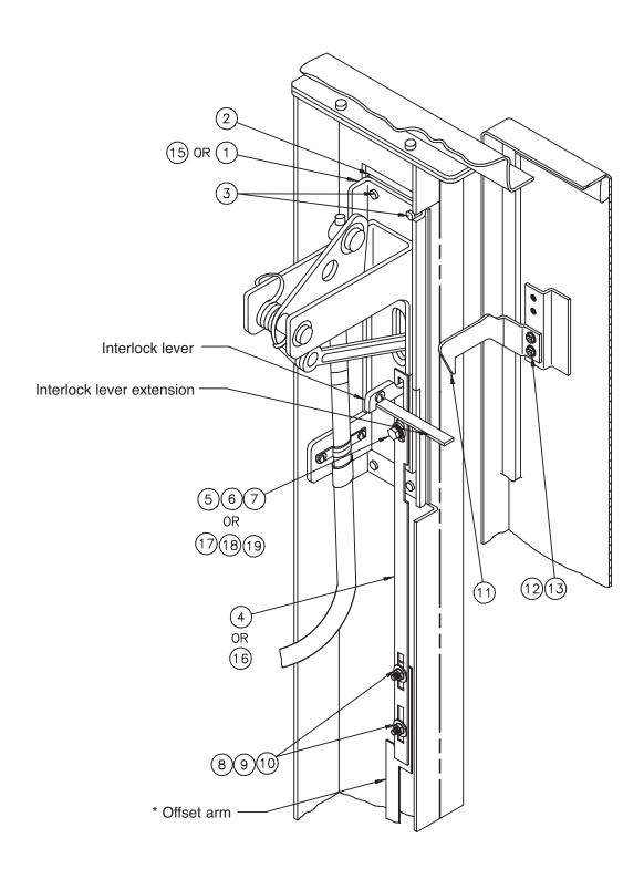
\* Parts of lock release mechanism
