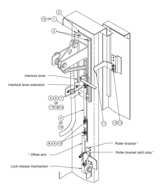
\* Parts of lock release mechanism
