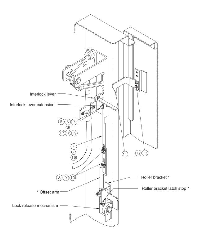
\* Parts of lock release mechanism
