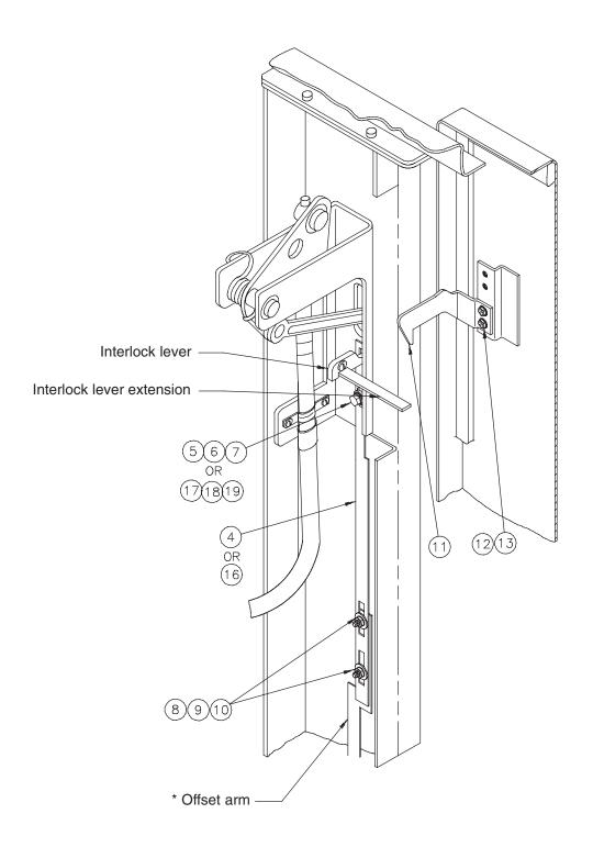
\* Parts of lock release mechanism
