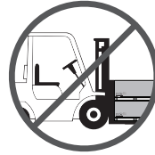
Crates stacked too high on forks lines.
