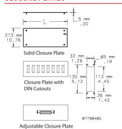
Closure Plates seal the ends of the cable entry cabinet. Made from 2,0 mm steel and finished with RAL 7035 textured gray polyester powder paint.
