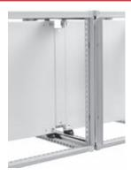
Provides a continuous panel surface in multiple-bay enclosures. The joining mounting plate is inserted between mounting plate of equal height. It can be installed from front or rear. Holes for grounding and mounting hardware are provided. Conductive mounting plates are unpainted galvanized steel.
