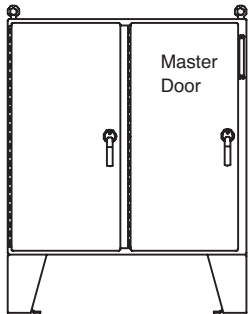
Two door enclosure with disconnect on right flange
