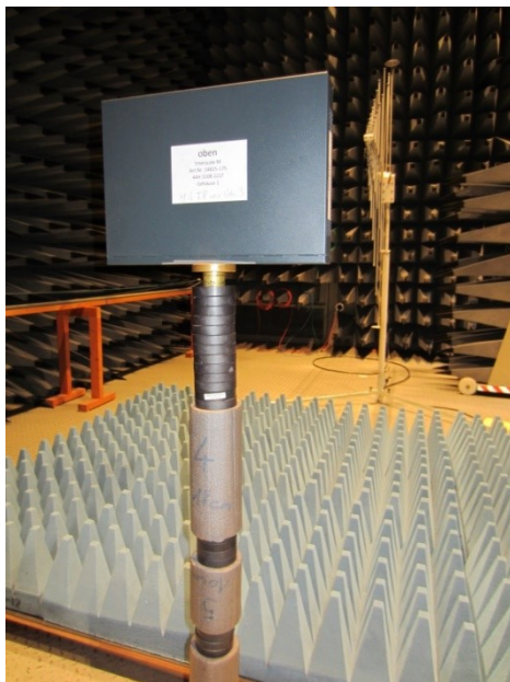
Fig. 5: Setup for the frequency range of 30 MHz - 1 GHz
