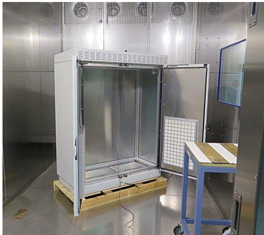
Cabinet after testing / Fans are running
