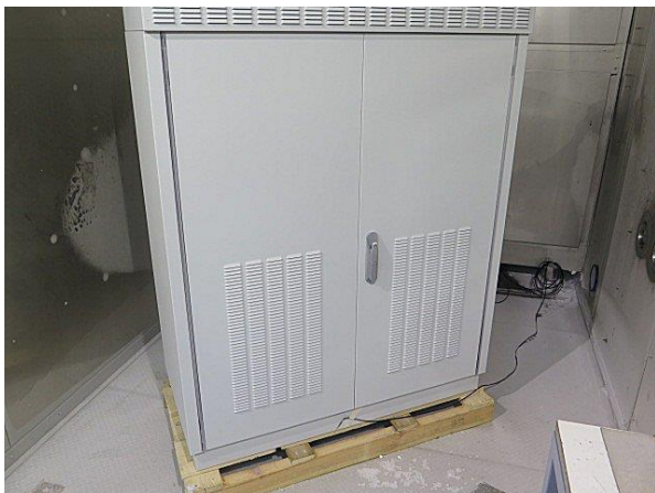
Cabinet at -45°C inside the climatic chamber
