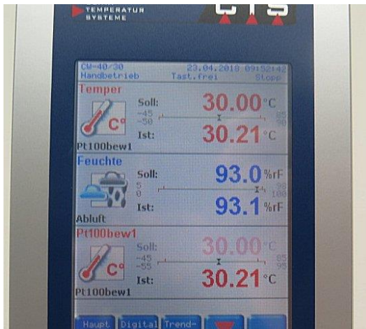
Temperature inside the climatic chamber
