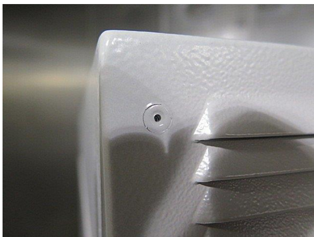
Crack around the rivet
