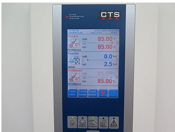
Temperature inside the climatic chamber
