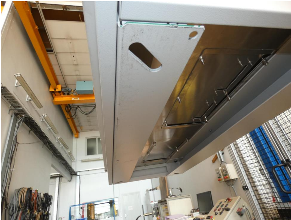
Photograph n°2 : Underside of the cabinet 29U after drop at 0.1m
