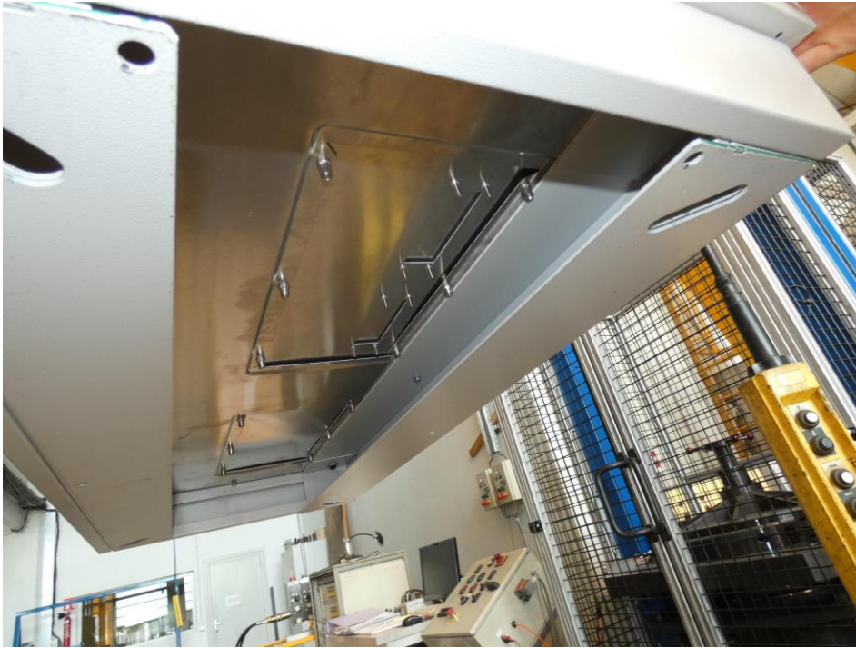
Photograph n°3 : Underside of the cabinet 29U after drop at 0.1m
