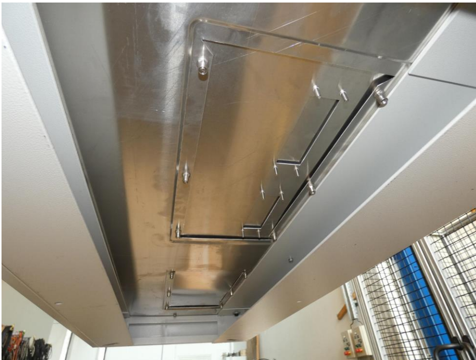
Photograph n°4 : Underside of the cabinet 29U after drop at 0.1m
