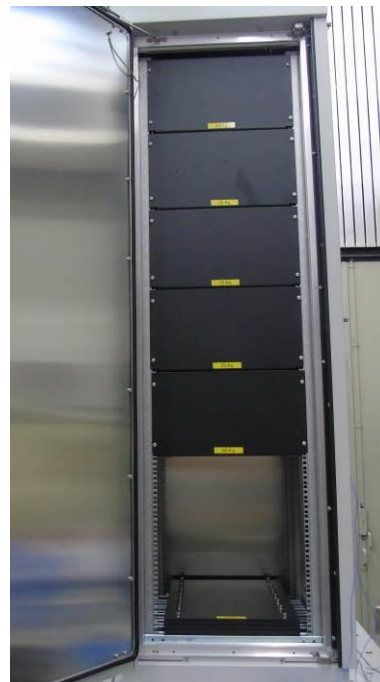
Fig. 23-4 EUT with dummy weights
