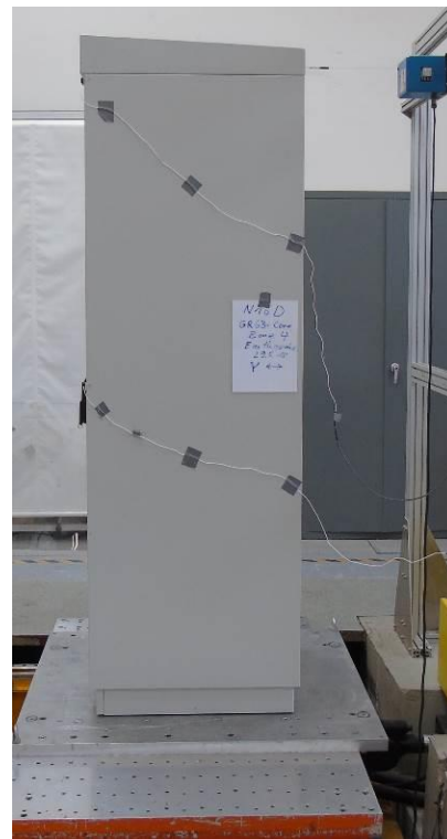
Fig. 23-8 Entire built-up for waveform testing (y-axis)
