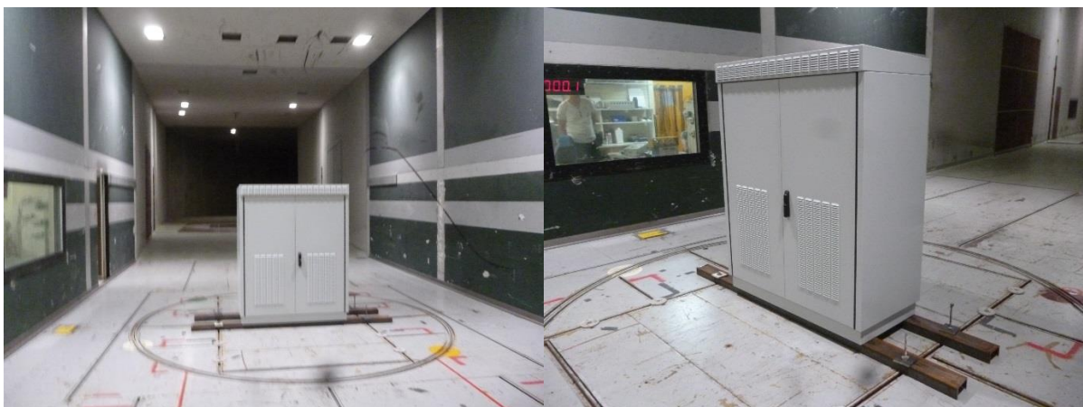
Figure 4: The cabinet in the high speed section of the climatic Wind Tunnel
