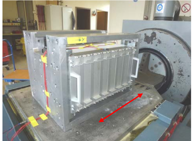
2: UUT in y-axis on slip-table
