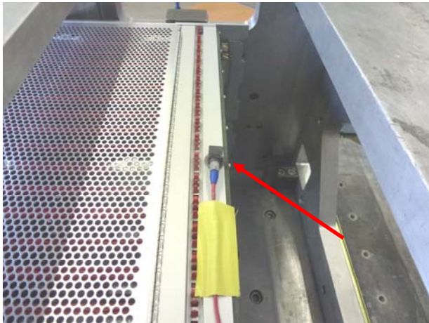
5: measuring point channel 4, back horizontal rail, top, center
