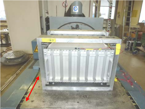
1: UUT in x-axis on slip-table
