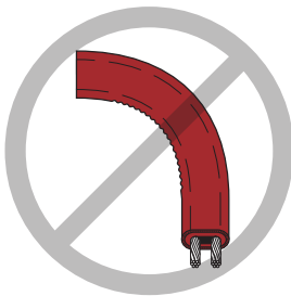
Figure 7: Bending the SC heating cable
