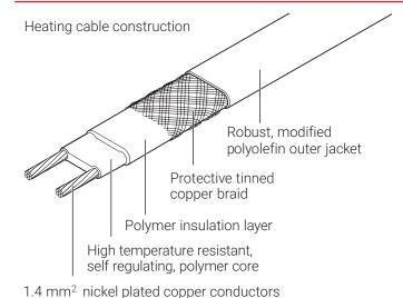
The nVent RAYCHEM FS-C10-2X self regulating heating cable protects pipes against frost damage. The cable is installed on the pipe under the insulation.
