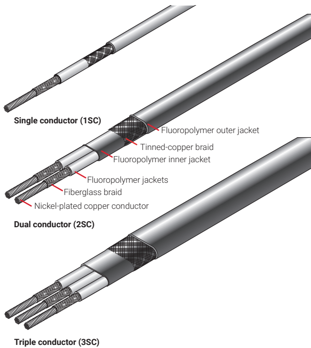
Heating cable construction
