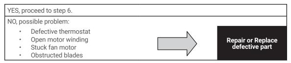
6. Carefully check the compressor for operation - motor should cause slight vibration, and the outer case of the compressor should be warm. Is the compressor showing signs of this?
