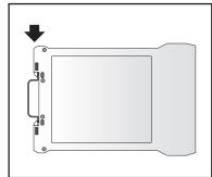
**REMOVAL:** Push the module upwards to disengage the clip, then rotate the module toward you.
