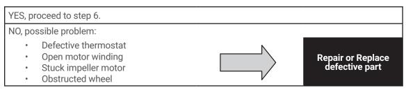
6. Carefully check the compressor for operation - motor should cause slight vibration, and the outer case of the compressor should be warm. Is the compressor showing signs of this?
