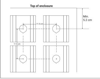
2. To mount the SSR at the outside of the panel drill a hole with the dimensions as marked on the drawing. Make sure that the notch is at the bottom of the hole drilled.
