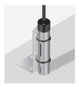
The FFS body should be secured to the mounting bracket via zip ties or some other removable retention mechanism. It may be desirable to move the FFS out of the way during equipment maintenance, either to protect it from damage or prevent a false alarm due to fuel spilled during maintenance activities. Therefore, the retention method used should allow easy removal and re-installation.
