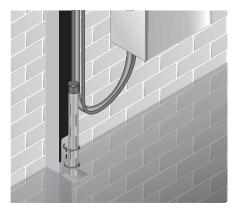
⚠ Warning: The FFS can be damaged if immersed in water and the water freezes. The sensor must be removed from the water prior to freezing (i.e. by draining the area or moving the sensor) or heating measures must be taken to prevent the water from freezing.
