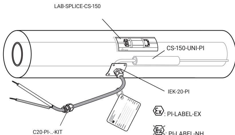
If used as a connection kit, follow the following steps for the termination of the PI cold lead cable in the junction box (optional, components are not included).
