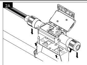
For the RayClic-PC power connection, fold up the four outer snaps, then position the connector over the snaps and press down.
