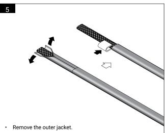
Place the metal clip over the base of the exposed braid.
