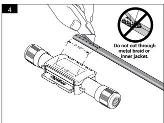
Score around and down the outer jacket of the heating cable 3 1/8 inches from the end.
