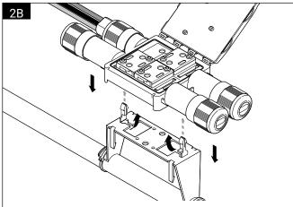
For the RayClic-PS powered splice and the RayClic-PT powered tee, fold up two center snaps, then position the connector over the snaps and press down.
