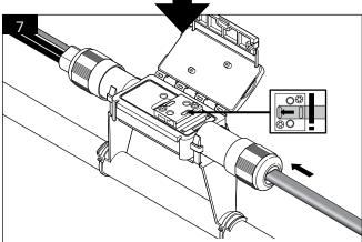
Insert prepared heating cable end into connector. Push until heating cable is fully inserted and end is visible through opening in connection cover plate.
