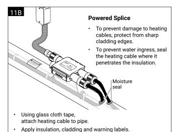
Terminate power wiring in user-supplied junction box.
