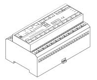
Remote Monitoring Module for Digital Inputs (RMM2-DI) provides digital input monitoring capability for the nVent RAYCHEM NGC-30 system. The RMM2-DI accepts inputs up to 15 digital inputs per module. Up to 247 RMM-DI modules can be connected to the nVent RAYCHEM NGC-30 system. The RMM2-DI module can be installed in ATEX / UKEx / IECEX Zone 2 hazardous area. For more details see the RMM2-DI datasheet.
