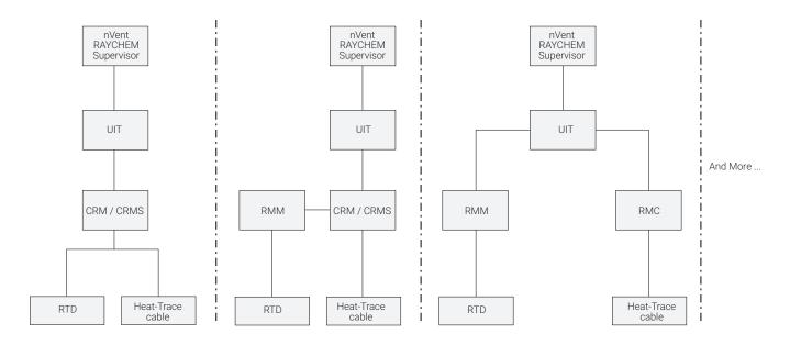
Examples of various nVent RAYCHEM NGC-30 configurations The following section gives an overview of the different components used in the nVent RAYCHEM NGC-30 system.
