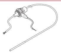
Mineral Insulated temperature sensor with M16 brass gland, installed on the sensor lead. Both are approved for use in hazardous area. (Sealing washer, locknut and earth tag are included)
