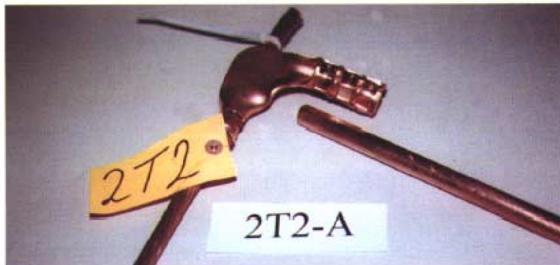
Figure 4: Typical Mode of Failure for Die Compression Type Connectors
