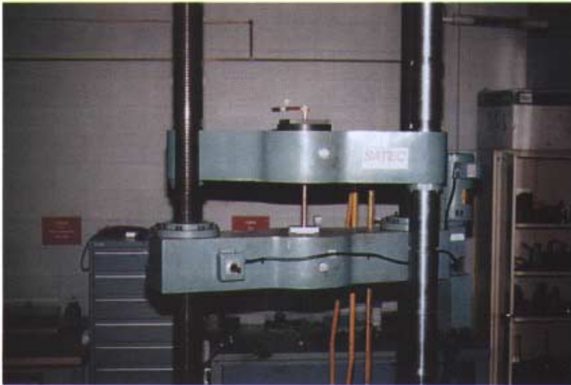
Figure 2: Typical Mounting of Connector for Mechanical Pullout Test
