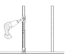
Set to desired height for box  $\mathbb{Q}$  . Align on stud. Attach screw through keyhole.
