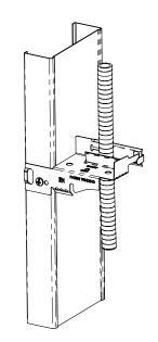
Bend side locking tab to secure cables
