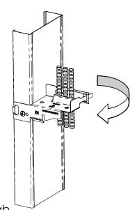
Bend tab. Engage back tab with locking tab.
