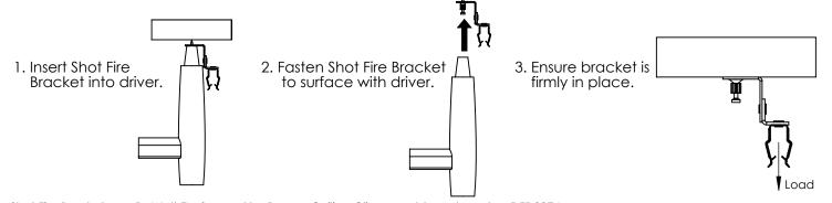
Shot Fire Bracket uses DeWalt Engineered by Powers Ceiling Clip Assembly part number DFD3374 Static load limits was established in normal weight concrete with a compression strength of 3,000 psi [20.68 MPa] and a 3-to-1 safety factor applied. Refer to DeWalt Engineered by Powers Ceiling Clip Assembly ICC-ES Evaluation Report ESR-2024 for the allowable load ratings in various substrate material and embedment depths.
