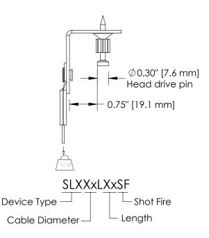
Uses Powers Fasteners, Inc. part number 50032. For minimum fastener embedment depths in steel or concrete, please consult www.powers.com.
