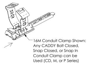
Conduit Clamp Registers on Extruded Pin
