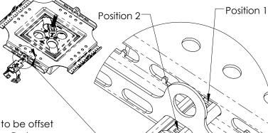
3 Conduits running close together will need clamps to be offset for fit. Push tab on clamp to release clamp off tab. Push clamp until clamp locks on tab in Postition 2.
