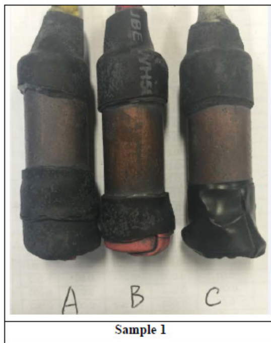
Appendix 4: Corrosion morphology for each of the replicate Cu-plated steels samples following 90 days exposure to GEM25A.
