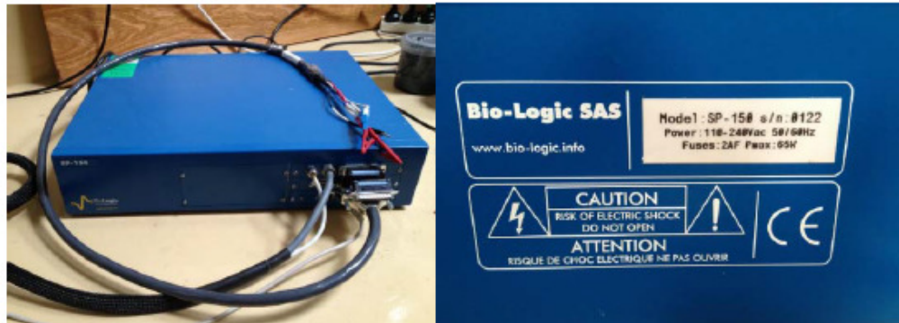
Figure 4. The Bio-Logic SP-150 potentiostat for LPR testing
