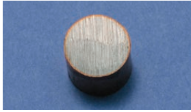
Cu-Bond Round Conductor cross-section
