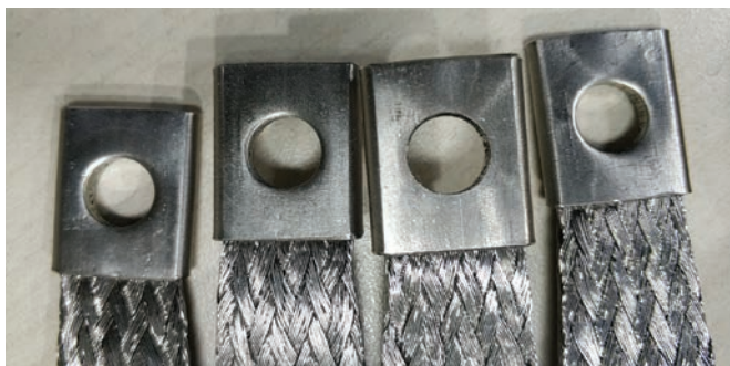
Figure 11 – Close-up shot of the nVent ERIFLEX CPI termination after vibration testing.
