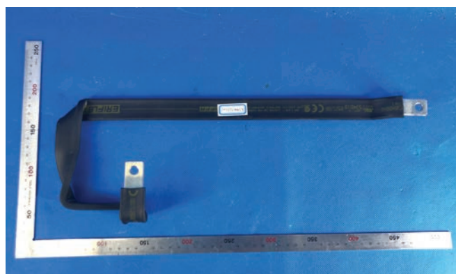
Figure 9 – nVent ERIFLEX Flexibar Advanced after testing
