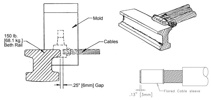
When using adaptor sleeves, let conductor protrude 1/8" beyond end of sleeve.
