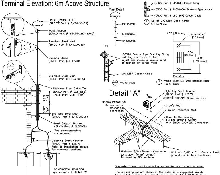
Two grounding systems required. One grounding system for each downconductor. The center ground rods to be minimum 50 FT [15M] apart.
