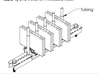
6) Install top rail with CABS insulators snapped in place.
