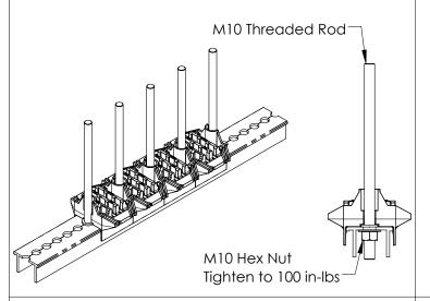
4) Mount to enclosure. Use Spacers to prevent deforming the aluminum profile when bolts are torqued.
