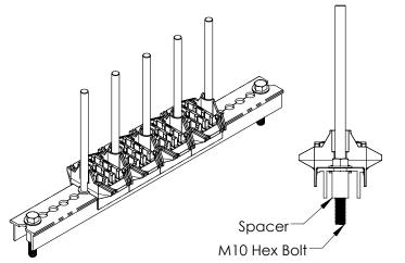
5) Install busbars. **Cut insulator tubing to length (see Table 1)** and install on threaded rods.
