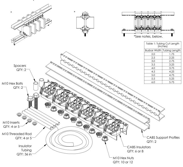
ONLY USE FASTENERS AND HARDWARE PROVIDED IN THE CABS HARDWARE KIT. Using fasteners and hardware that is not included may compromise performance and will void warranty. \*Busbars not included. Product is NOT shipped assembled.
