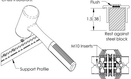
2) Install CABS insulators on Bottom Support Profile. Repeat for Top Support Profile.
