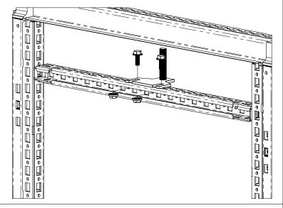
Step 2 - Attach assembly to enclosure or brackets. Reference Instruction Sheet IP 8347 for CABS assembly details. Tighten bolts as
