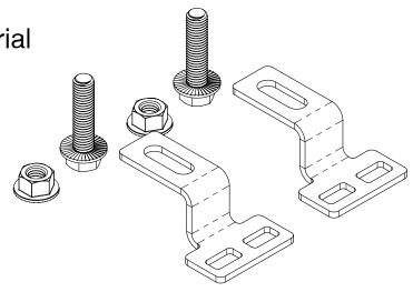
1) Attach bracket to enclosure frame in the desired orientation using nVent HOFFMAN BVM6.
