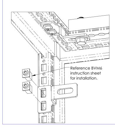
2) Fasten support rails to bracket using M10 Hex Bolt and M10 Hex Nut. Reference instruction sheet IP8347 for CABS system installation.
