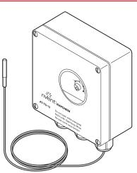
nVent RAYCHEM AT-TS thermostats provide temperature control in safe area. The temperature set point can be checked through a window in the lid. LED's are providing an indication when cables are energized (Heating ON) or when the temperature sensor is defect (sensor break or sensor short-circuit).
