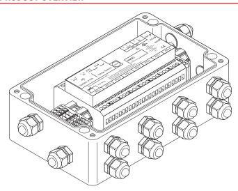
The Remote Monitoring Modules (RMM2) provide temperature monitoring capability for nVent RAYCHEM NGC controller family. The RMM2 accepts inputs from up to eight Pt 100 temperature sensors that measure pipe or ambient temperatures in a heat-tracing system. Multiple RMM2 units communicate with a single nVent RAYCHEM NGC User Interface Terminal (nVent RAYCHEM NGC-UIT) providing centralised monitoring of temperatures.
